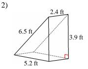
$V = 0.5x5.3x4.0x3.0 = 31.8 \text{ in}^3$ A = (5.3x4.0)+((5.3+5.3+4.4)x3.0) = 66.2 in<sup>2</sup>  $V = 0.5x5.2x3.9x2.4 = 24.3 \text{ ft}^3$ A = (5.2x3.9)+((5.2+3.9+6.5)x2.4) = 57.7 \text{ ft}^2
